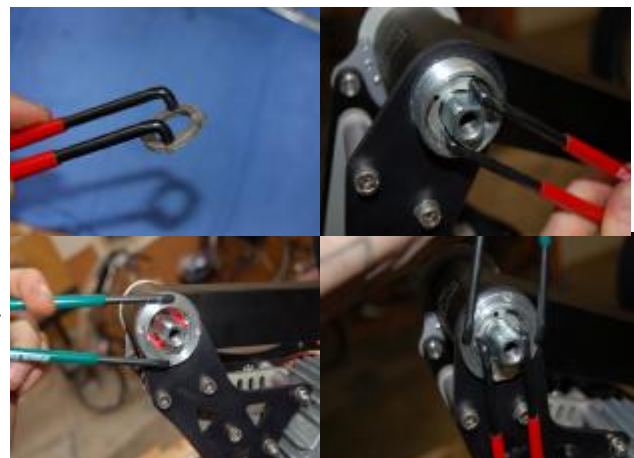
(6) Adjust Cup and Lock-ring Install
