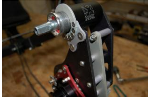
(4A) Installing New Bottom Bracket
