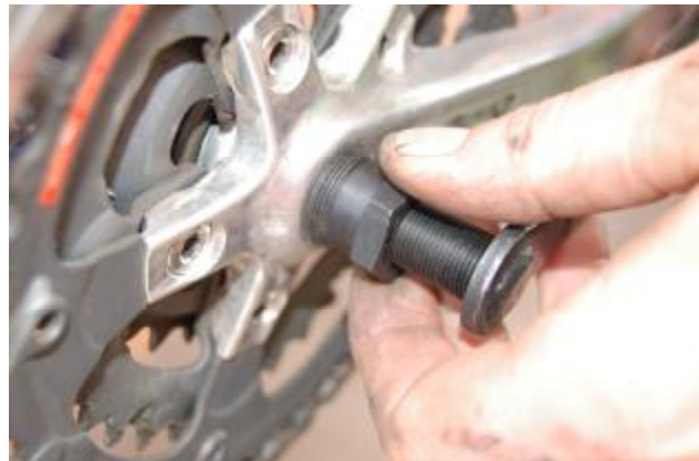
(2) Removing Crank with Crank Puller
