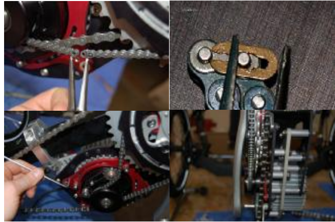
(8) Installing Chain, and Align Using Set Screws
