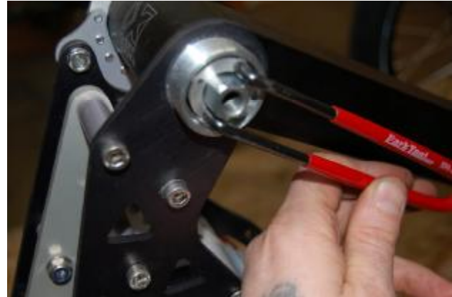
(4D) EMtnD Hanging from Collar on Bottom Bracket, Using Proprietary Tool.
