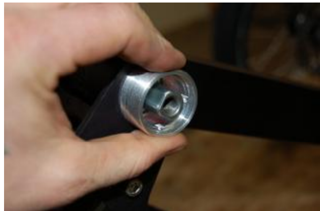
(4C) Left Side BB Nut Partly Installed
