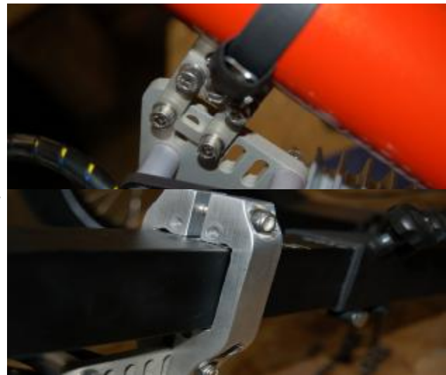
(5) Clamps Installed On Frame
