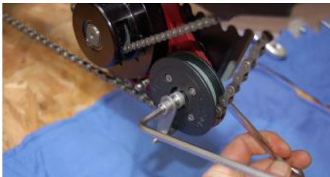
(7) Installing Crankset, Drive Chain, and Return Chain Idler
