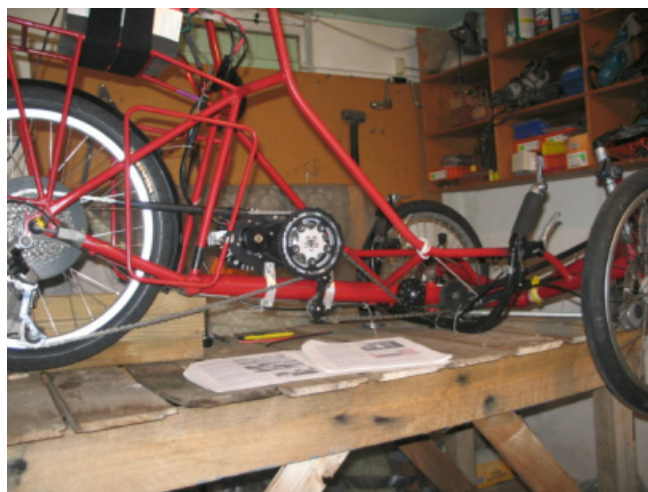
The chain has a tensioner for the front run as well as the back. Motor sits neatly under the seat of the touring Greenspeed trike.
